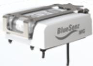
**WirelessGate** is a Radio Frequency (RF) communication device. It collects data from the various sensors on-board the ship (e.g. WinchSenz, NetSenz) and then transfers this data via the BlueTraker VMS device to the database server on land.
